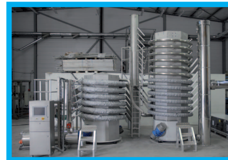
500 kg/h steam sterilization unit for spices
