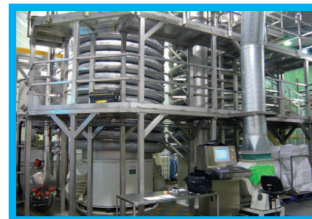
2250 kg/h nut pasteurization unit
